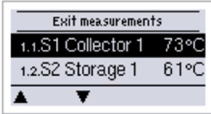
The menu "1. Measurement values" serves to display the currently measured temperatures.
