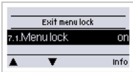
Menu "7. Menu lock" can be used to secure the controller against unintentional changing of the set values.
