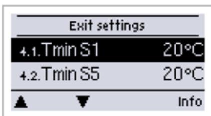
The necessary basic settings required for the control function are made in menu “4. Settings”.
